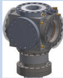
reactors with inspection ports
