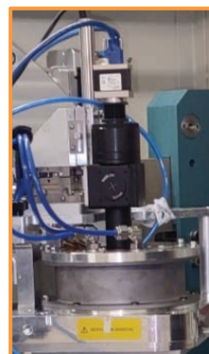
Custom reactors. Shown is a reactor with beryllium side walls for use on synchrotron SXR setups.
