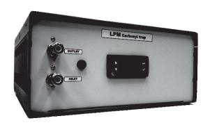
The CarbonylTrap has an optimal conversion using pure Cu-shots in Cu-tubing. This copper tubing of the high-temperature stage prevents the reformation of any nickel carbonyls.
