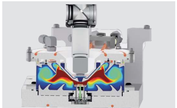
Cross sectional view of the reactor showing an optical microscope system with objective on top, sample heater stage at the bottom and the reactor volume with the special designed structures to deflect the gas flow. The color coding indicates the Cu vapor distribution in the reactor for a given gas flow rate and when a Cu substrate is heated above its melting point.
